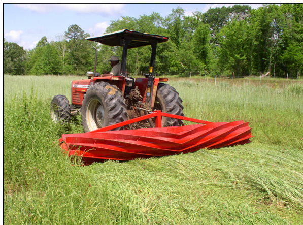
A specially designed roller crimps the rye stem and lays it flat. The next crop is no-tilled into the cover.
